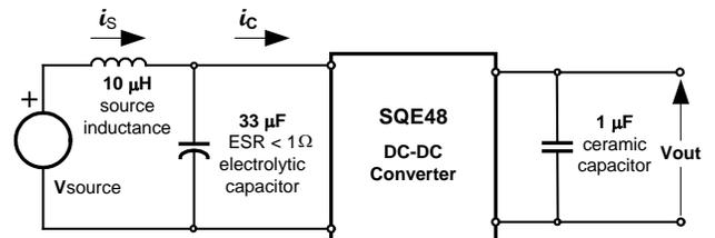
**Fig. 1.8V.12:** Test setup for measuring input reflected ripple currents,  $i_c$  and  $i_s$ .
