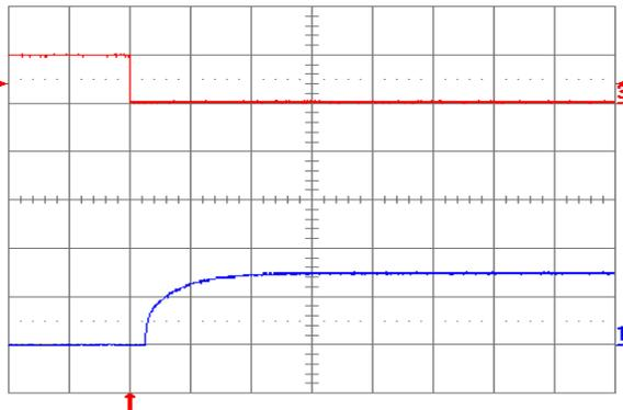
**Fig. 1.5V.7:** Turn-on transient at full rated load current (resistive) with no output capacitor at  $V_{in} = 48\text{ V}$ , triggered via ON/OFF pin. Top trace: ON/OFF signal (5 V/div.). Bottom trace: Output voltage (1 V/div.). Time scale: 2 ms/div.
