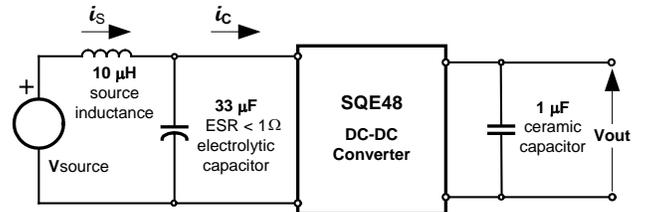
**Fig. 2.5V.12:** Test setup for measuring input reflected ripple currents,  $i_c$  and  $i_s$ .
