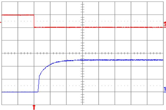
**Fig. 2.5V.7:** Turn-on transient at full rated load current (resistive) with no output capacitor at  $V_{in} = 48\text{ V}$ , triggered via ON/OFF pin. Top trace: ON/OFF signal (5 V/div.). Bottom trace: Output voltage (1 V/div.). Time scale: 2 ms/div.
