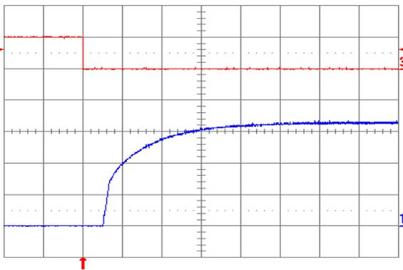
**Fig. 3.3V.7:** Turn-on transient at full rated load current (resistive) with no output capacitor at  $V_{in} = 48\text{ V}$ , triggered via ON/OFF pin. Top trace: ON/OFF signal (5 V/div.). Bottom trace: Output voltage (1 V/div.). Time scale: 1 ms/div.
