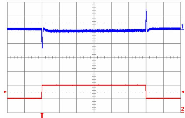
**Fig. 3.3V.10:** Output voltage response to load current step-change (10 A – 20 A – 10 A) at  $V_{in} = 48\text{ V}$ . Top trace: output voltage (100 mV/div.). Bottom trace: load current (10 A/div.). Current slew rate: 5 A/ $\mu\text{s}$ .  $C_o = 470\ \mu\text{F POS} + 1\ \mu\text{F ceramic}$ . Time scale: 0.2 ms/div.
